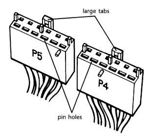
There is one 12-pin power supply socket on the right side of the main system board (toward the back) that holds both of the power supply connectors, as shown below.
